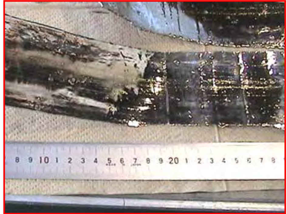
Ti-based BMG large plate with width of 80 mm, length of 200 mm
