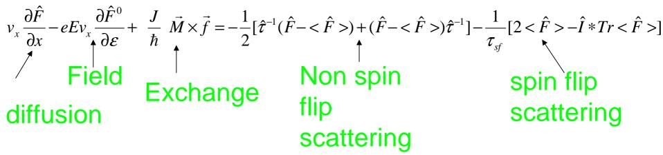
Solution of Boltzmann equation across interface between *noncollinear* magnetic layers.
