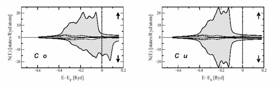
Figure 2.6: Spin-projected densities of states for Co and Cu; the differently shaded grey areas indicate the amount of s, p and d states.
