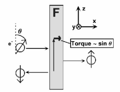
FIG. 1. Schematic of exchange torque generated by spin filtering. Spin-polarized electrons are incident perpendicularly on a thin ideal\_freetoncagatia\_seco\_Sain\_filtaric\_seconcagations.
