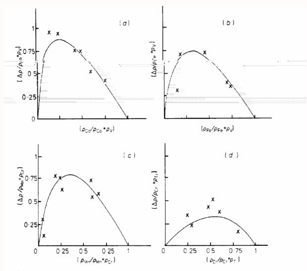
**Figure 1.** Deviations from Matthiessen's rule in Ni based ternary alloys (relative deviations grainst relative constituines) 491 NiCoV 491 NiEv 471 NiMoC 401 NiCrTi The full curves are calculated from expression (19) with the values of  $\alpha$  listed in table 1.
