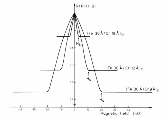
FIG. 3 Magnetoresistance of three Fe/Cr superlattices at 4.2 K. The current and the applied field are along the same [110] axis in the plane of the layers.
