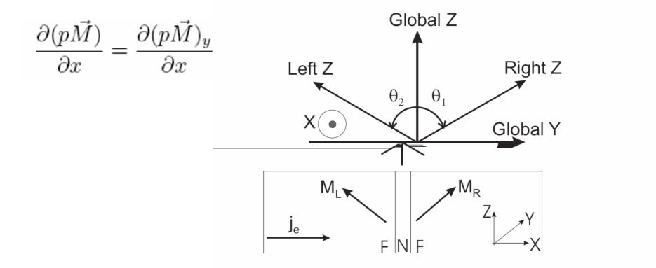
3. 1: Coordinates. The current is in x or growth direction in this multilayer. The magnetization FIG ections of the two ferromagnetic layers  $M_L$  and  $M_R$  are in y-z plane. The global z direction is direction is the sen in between  $M_L$  and  $M_R$ .
