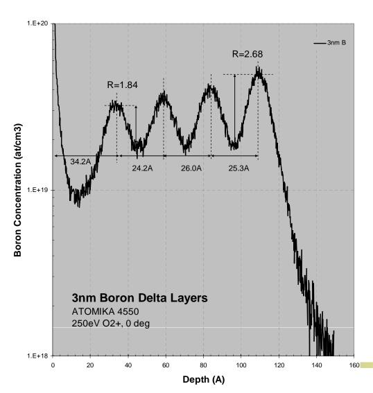
B spikes separated by 3 nm using SIMS with trailing edge slope > 2 nm/dec;
