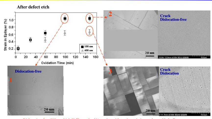
Dislocation-free 100nm thick Si film under 1% tension with strain variation undetectable by Raman
